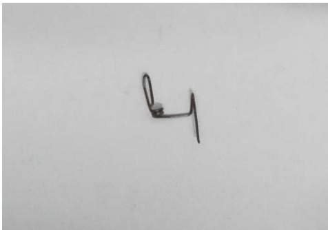
Figure 3 Showing Beggs rotation spring.
